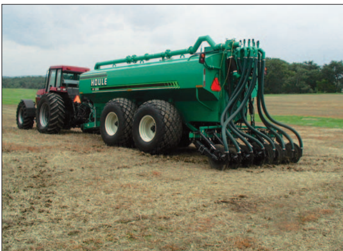
FIGURE 22. Manure injection limits ammonia losses and odor from liquid manure in no-till.
